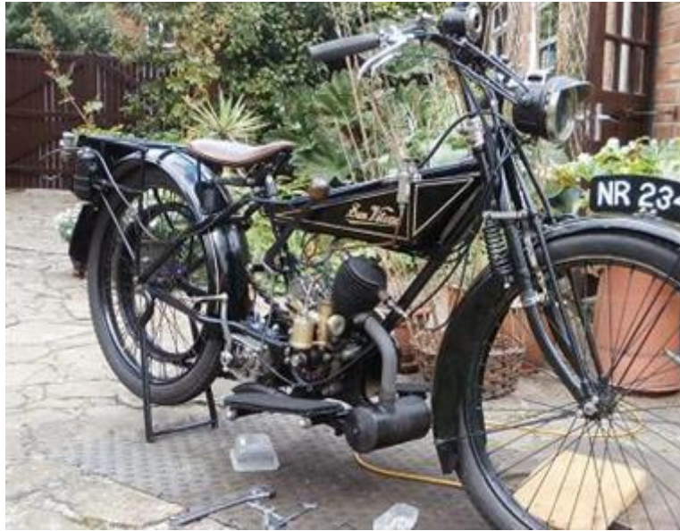
A 1922, 268cc Sun motorcycle fitted with a two-stroke Day engine
